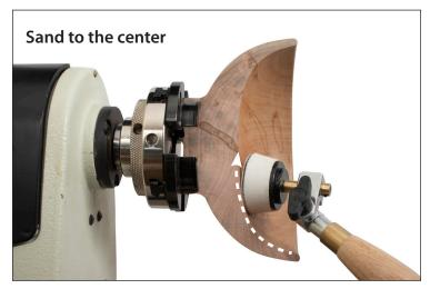
Once you reach the center of the rotating project, lift the sander off the work surface and start sanding again at the rim of your project. Do not sand past the center of your project.
