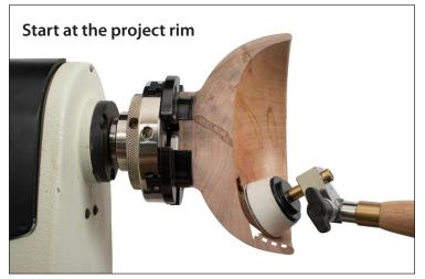
With your project mounted to your lathe and rotating at a slow speed and with light pressure, start working the sander from the rim. Remember to keep the sander moving.
